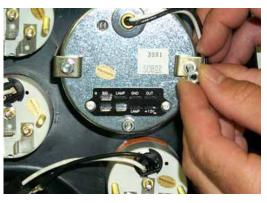
STEP 6: Install mounting clips on tachometer & speedometer.
