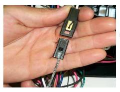
STEP 11: Plug each lamp power wire (white) into the mating connectors on each grey wire (DASH LIGHTS) on the new harness.
