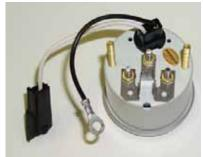
STEP 4: Install appropriate lamp socket pigtails into the speedometer & tachometer.
