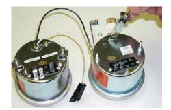
STEP 5: Insert gauges into housing, in locations shown.
