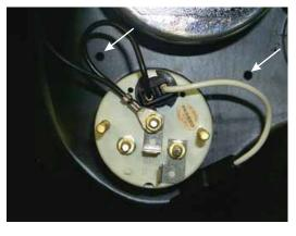
STEP 7: Drill 4 mounting holes for LED's, using 5/32" drill bit, at desired locations. Insert LED's in hole from front of panel.
